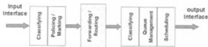
Fig. 2. Forwarding process within a router
